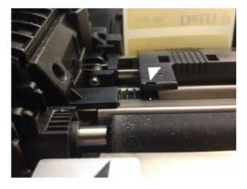
Now push the media guide to the left, pushing the two sensors along with it, for about 0.5 cm.
