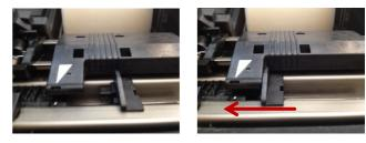
4. Now you can move the Media guide back into position and setup the printer. Make a print of one of your label layouts to test that everything works as expected.
